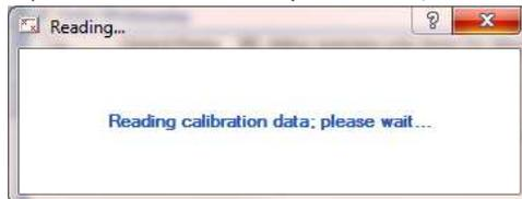
If valid calibration data is held in the controller it is utilized otherwise calibration data held locally is used. If Calibration settings (no. of points, margin etc) are also held in eeprom (space permitting) they are used as stored. If they are not held then the calibration values defined in the UPDD Console need to match the eeprom data reference points.
